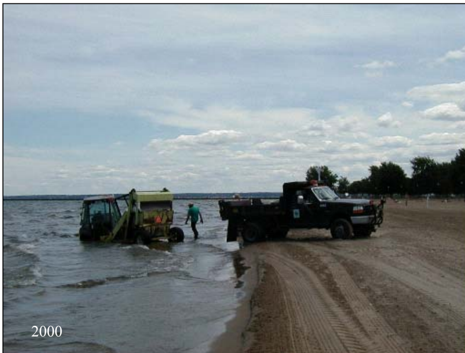
Parks Department Rake - Fine teeth on a drum deposits material into a hopper, used mainly for the material on the sand and very shallow. Works pretty well, but its efficiency is limited by the hopper size.
